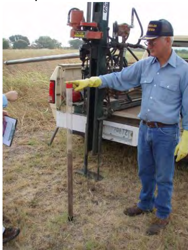
USDA soil core failure from hard dry soil – note that only half the one meter core sleeve has soil
