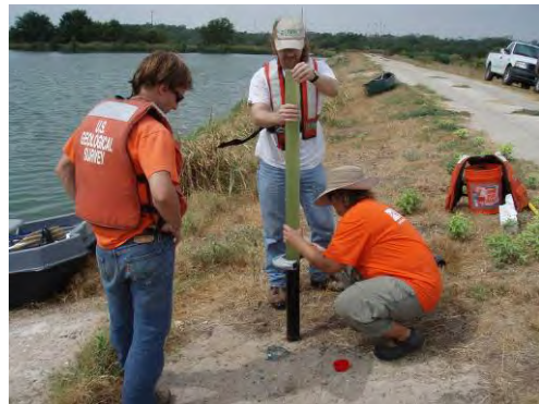
USGS cutting a sediment core removed from Pond 1 East
