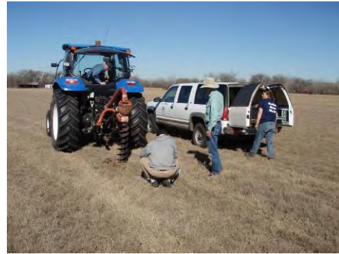
Soil Sampling with auger Tractor operator Steve Hall
